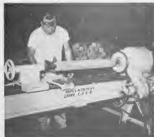
DOWELS FORMED in greenheart are inserted in the Carpenter Shop and then driven into openings in new timbers where bolts had been driven through. Glued and sawed flush, the result is a closed, smooth finish on the timber's outside side. This was done 4000 times along the length of the pier.
